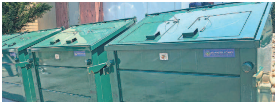
Gatlinburg's new dumpsters automatically latch in a manner that prevents bears from accessing them. The $2.8 million investment has had an immediate impact on bears' ability to access human food in the city. PROVIDED BY THE CITY OF GATLINBURG
