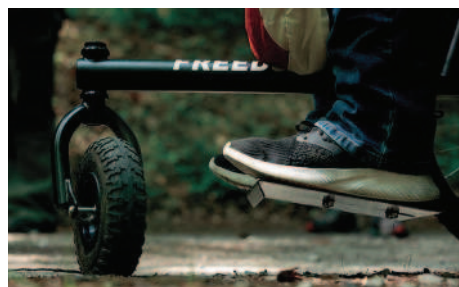
A mix between a manual wheelchair and a mountain bike, the park's GRIT Freedom Chairs feature a third wheel in front for stabilization. Users can propel themselves by pumping the hand levers, or they can receive a push from behind.
