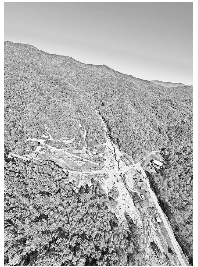
Damage caused by mudflows into Flat Creek near the Garren Creek Fire Station, shown on Oct. 17, 2024. Some of the initiating landslides are visible in the distance, upper left of photo. PROVIDED BY UNITED STATES GEOLOGICAL SURVEY
